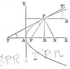
Let PT be a tangent to the parabola at P, and let PF be the radius vector drawn to the point of contact.
