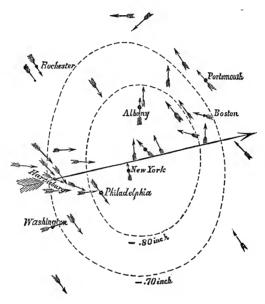
which the barometer sunk eight tenths of an inch below the mean, and the larger oval shows the area within which the barometer was depressed seven tenths of an inch. The long arrow represents the direction in which the storm advanced, while the short arrows show the observed direction of the wind at nearly forty different stations.
