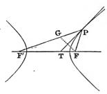
190. To draw a tangent to the hyperbola through a given point of the curve. Let P be the given point; draw the radii vectores PF, PF'; on PF' take PG equal to PF. and draw FG. Draw PT perpendicular to FG, and it will be the tangent required, for it bisects the angle FPF'.
