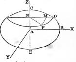
Hence  $ND^2 = \frac{a^2b^2 - a^2z^2}{b^2}$ . But  $ND^2 = NP^2 = NM^2 + MP^2 = x^2 + y^2$ ; hence  $x^2 + y^2 = \frac{a^2b^2 - a^2z^2}{b^2}$ , or  $b^2(x^2 + y^2) + a^2z^2 = a^2b^2$ ,
