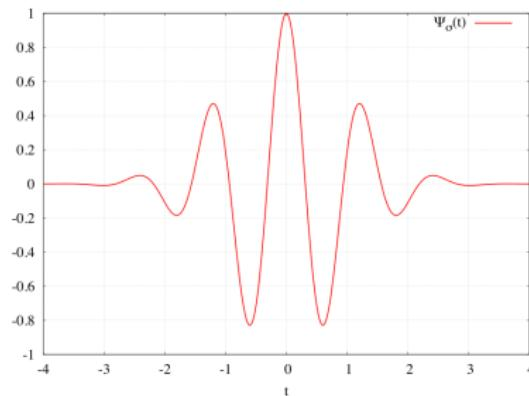
“A wave-like oscillation with an amplitude that begins at zero, increases, and then decreases back to zero”
